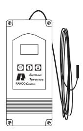
Though our evaporator section will operate at any ambient temperature above freezing, some customers want the machine to shut down before reaching freezing ambient temperatures. We supply an optional thermostat to do this. This control can also be used as a high temperature cutout in high ambient locations as in our south-western states. It operates with the bin control to shut the machine down. The AMBER pilot light will turn on as when the bin is full.
