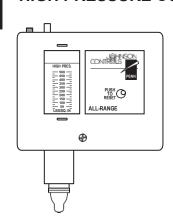
All currently manufactured machines no longer use the dual pressure switch, but two separate high and low pressure switches. Should the machine experience a high-pressure condition, the high pressure switch opens, and all functions of the machine will stop. Ther machine will not re-start until the reset button on the switch is pressed.
