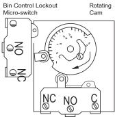
**Primary** Micro Switch Bin thermostats, mechanical bin controls, and remote OFF/ ON switches may be activated at any time during the freeze and harvest cycles. Machine operation will continue upon opening any of these controls, and machine shutdown will be delayed until the roller on the bin control lockout micro switch is in the detent position of the cam.
